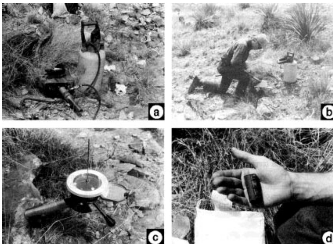
Figure 4.2 Core sample collection procedures. (a) Portable gasoline-powered drill with diamond drilling bit; a pump can is used to force cooling water through the drill bit. (b) Unskilled laborer drilling a core. (c) Orientation stage placed over in situ core. Notice the inclinometer on the side of the orientation stage; the magnetic compass is under a Plexiglas plate; the white ring on the Plexiglas plate is used to measure the azimuth of the shadow cast by the thin rod perpendicular to the plate. (d) Core sample with orientation markings.
