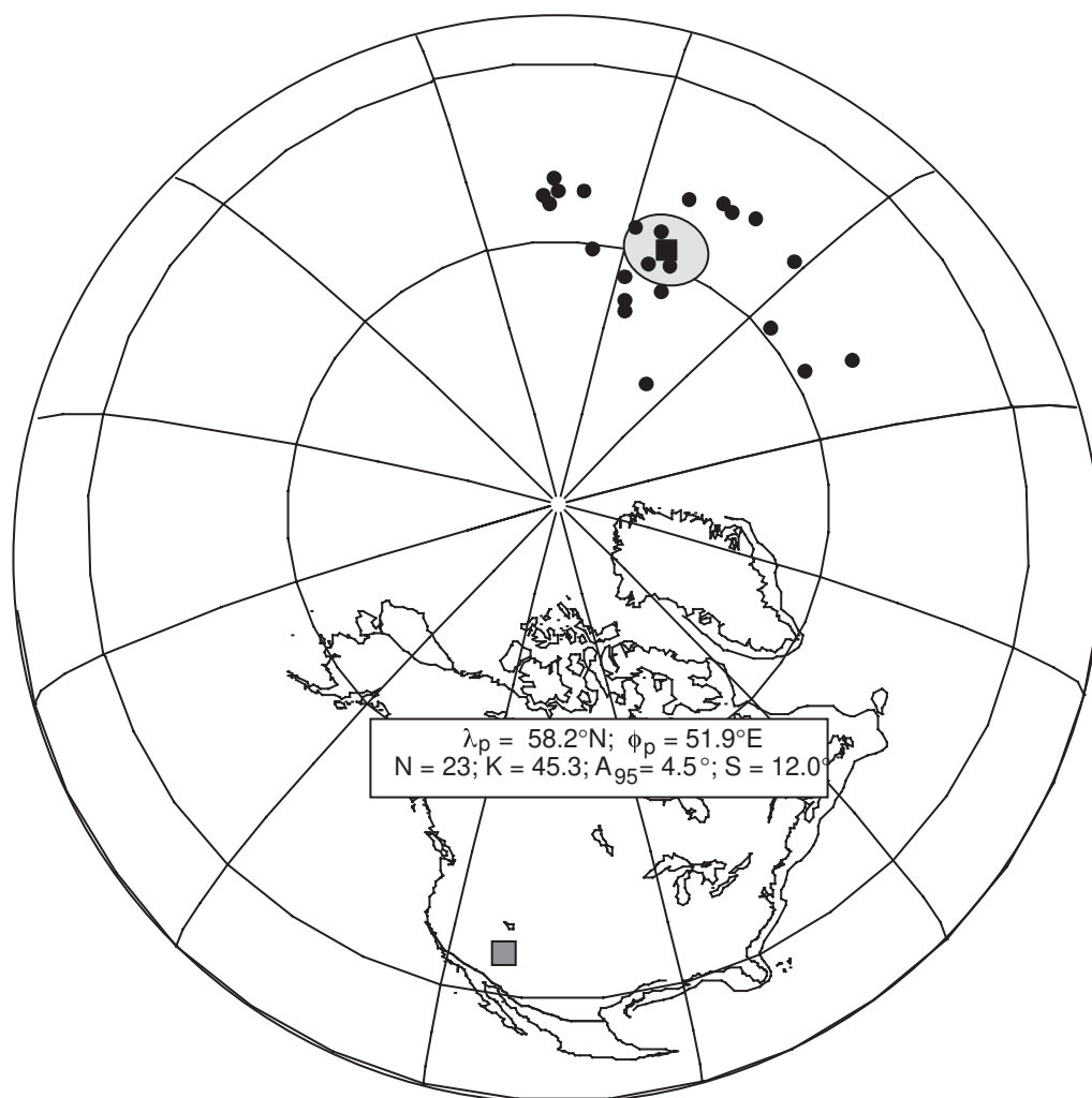
Figure 7.3 Paleomagnetic pole from the Moenave Formation. Solid circles show the 23 site-mean VGPs averaged to determine the paleomagnetic pole shown by the solid square; the stippled circle about the paleomagnetic pole is the region of 95% confidence with radius A_{95} ; the region of sampling is shown by the stippled square; the inset gives the location of the paleomagnetic pole along with statistical parameters.
